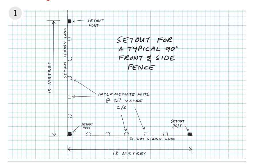
**Plan:** the fencing project on graph paper before proceeding. Check that the fence lines are correctly positioned in relation to the boundary and/or survey pegs. Ensure the fence and fence height conform to local council bylaws and subdivision covenants
