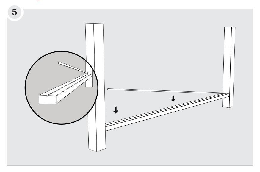
Trim the bottom rail infill bead to the length of the bottom rail. Fit the bottom rail infill bead into the centre groove of the bottom rail (tapered side up). Avoid excessive bending of the infill bead to avoid breakage.
