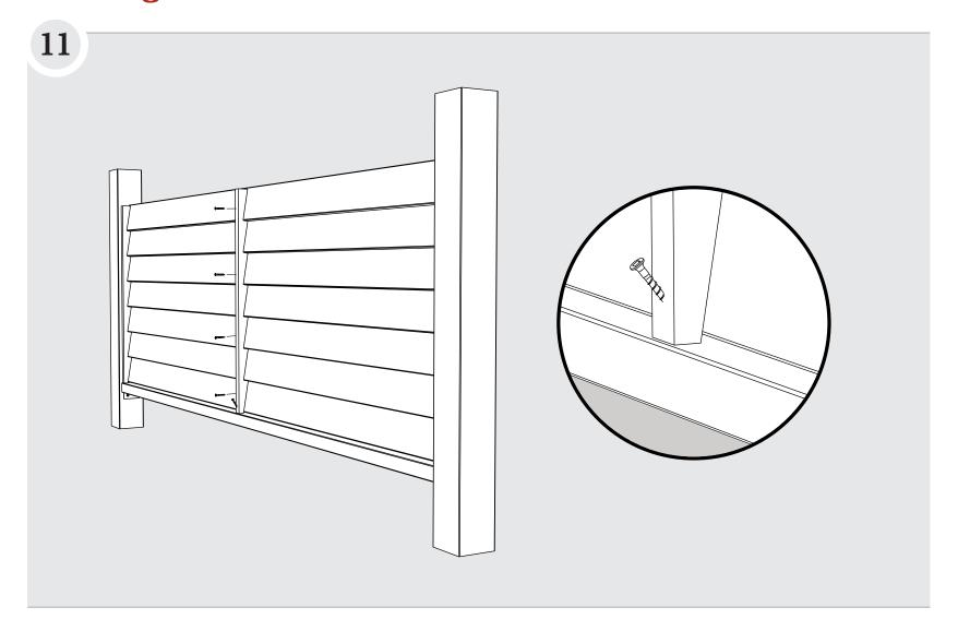
Trim and install the 42x36mm centre scriber on the rear side. Screw fix into every second fence board.
