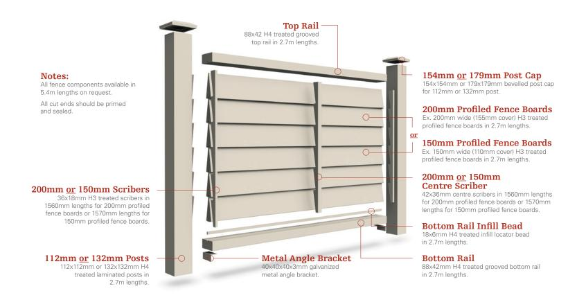
All components are manufactured from clear exterior treated finger-jointed radiata pine and are machine primed and undercoated with a two-coat oil based coating system.
