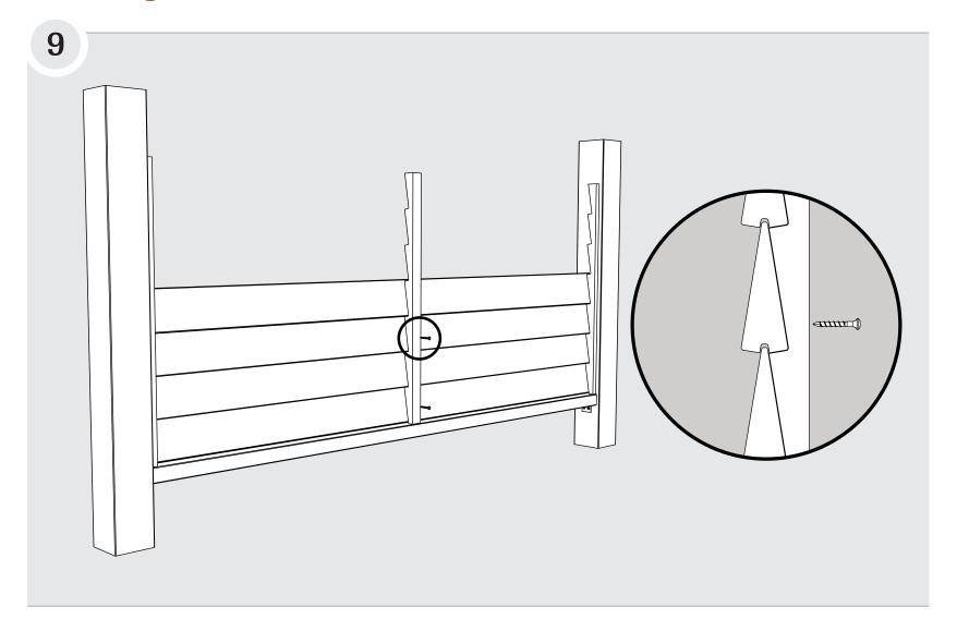
Trim the 42x36mm centre scriber to match 18mm side scribers already installed. Install centre scriber on front side after the fourth fence board is in place.
