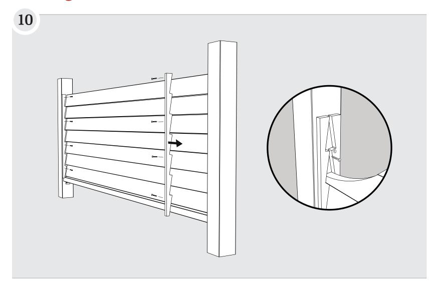
Trim and locate the rear set of 18mm side scribers to the reverse side of the fence and secure to the post as per step 7. Apply hand pressure to the scriber so it seals firmly against the fence boards.
