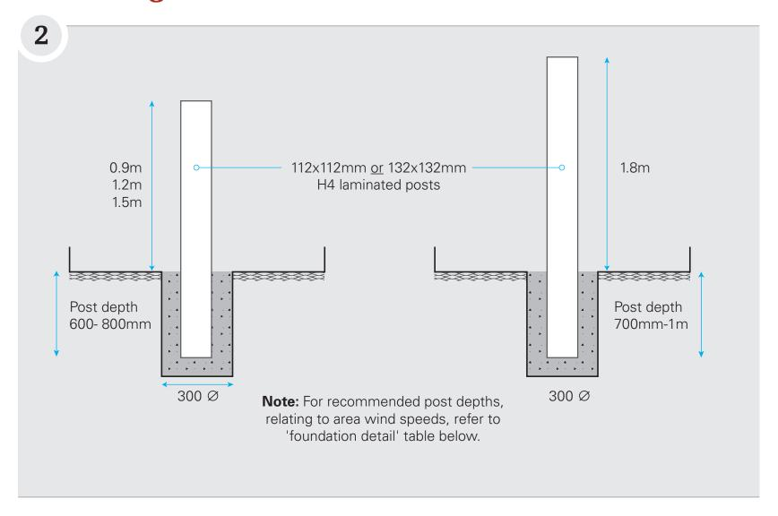
**Setout:** Peg out, excavate and concrete-in a post at either end of the fence line. Ensure posts are accurately positioned and plumb as these determine the accuracy of the fence line.
