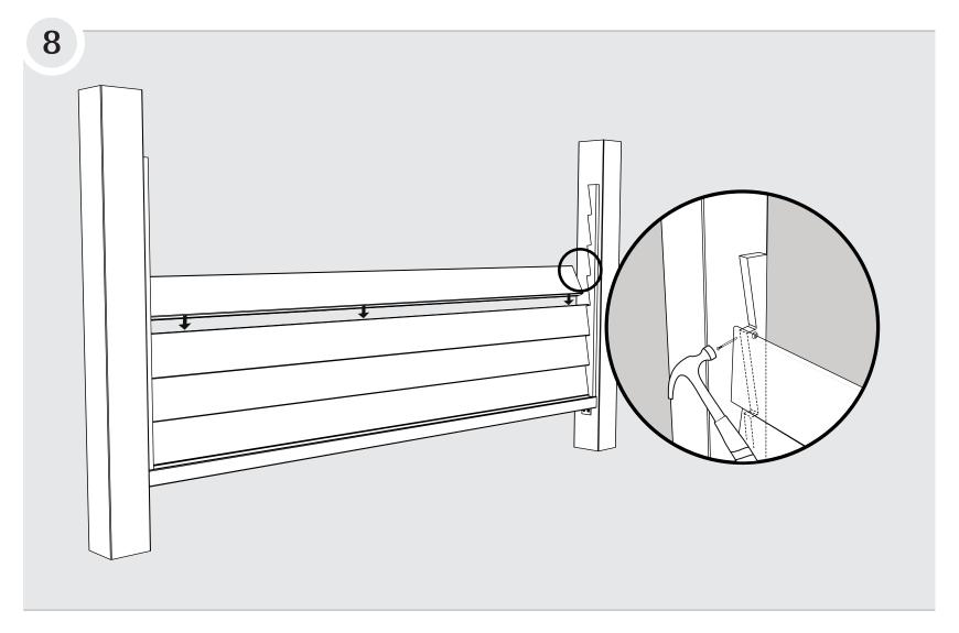
Trim and stack three more fence boards to the required height by fitting into the 36x18mm scriber. From the rear side, lightly pin through the top of the fence board to the scriber. Once set nail/punch pins flush with the profiled fence board.
