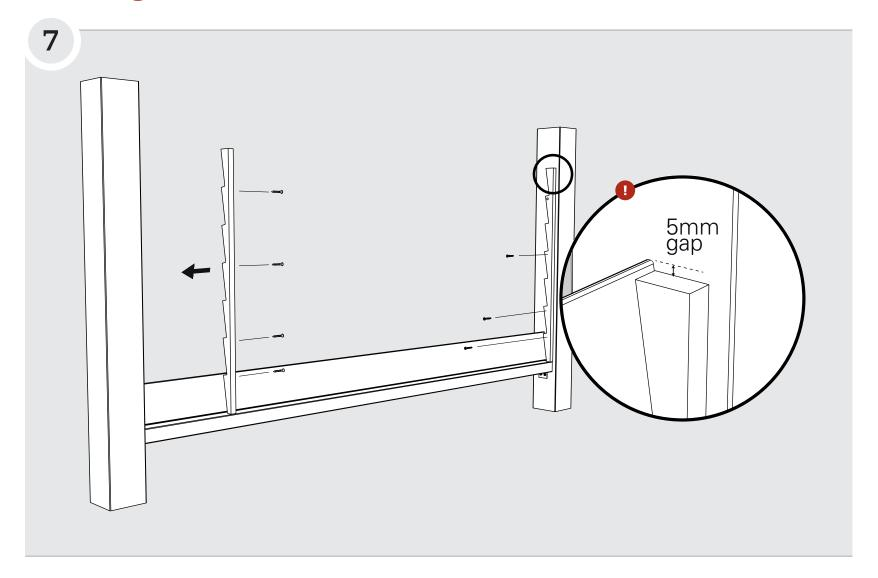
Measure, trim and locate one set of 36x18mm scribers to the front side of the fence. Fix scriber to the post with 10 gauge (40mm) stainless steel raised head screws at the top and bottom, and as required between.
