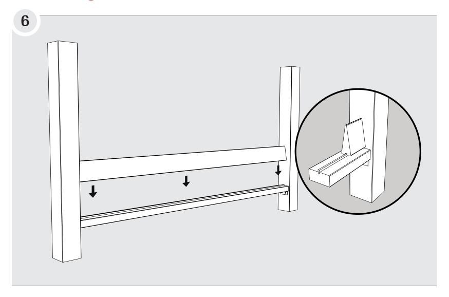
Trim the first fence board to fit. Install only the first fence board over the infill bead and bottom rail. This step assists in setting the scribers in the correct position.
